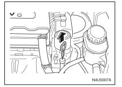
Use the engine oil dipstick to check the oil level. The dipstick's handle will be a yellow ring. See "Engine Compartment Overview" in this section for the location of the engine oil dipstick.
